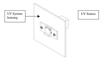
Figure 13-Locator Kit-Internal Mount on UV System
