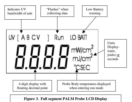
The following section goes over the various displays the user will see when the PALM Probe is used. Button or Membrane Switch action is described in the box on the left with a diagram of the PALM Probe LCD on the right.
