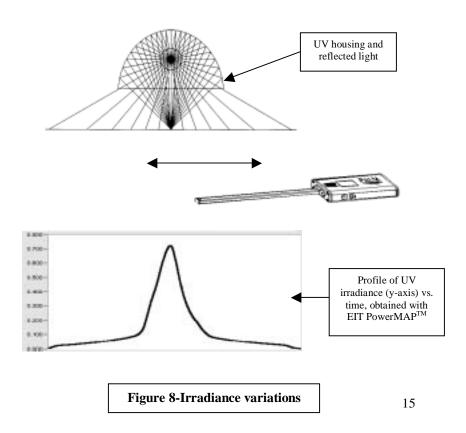
Variations in irradiance may also be seen when the PALM Probe is moved along the length of a UV bulb in addition to moving the Probe in and out of the focus of the UV lamp.
