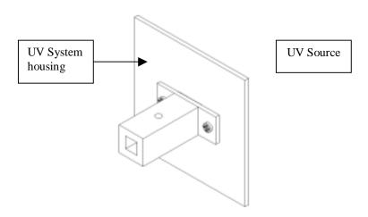
Figure 12-Locator Kit External Mount on UV System
