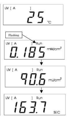
To stop collecting data, push the RUN/STOP button. Display stays on the unit value that was last on the LCD screen while collecting data.
